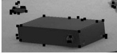
Fig. 2.10. The SUSAN operator has detected a set of gray value corners shown as black squares. We find all those gray value corners included which are characteristic for the three-dimensional object boundary.
